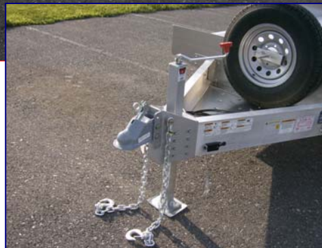
Heavy Duty Top Wind Jack With Drop Leg And Std. Adjustable Hitch Assembly
